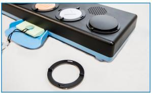
twist and lift. Always replace the ring at the base of the button switch to cover up the slots: This prevents dust and debris from getting into the circuitry of the player.
