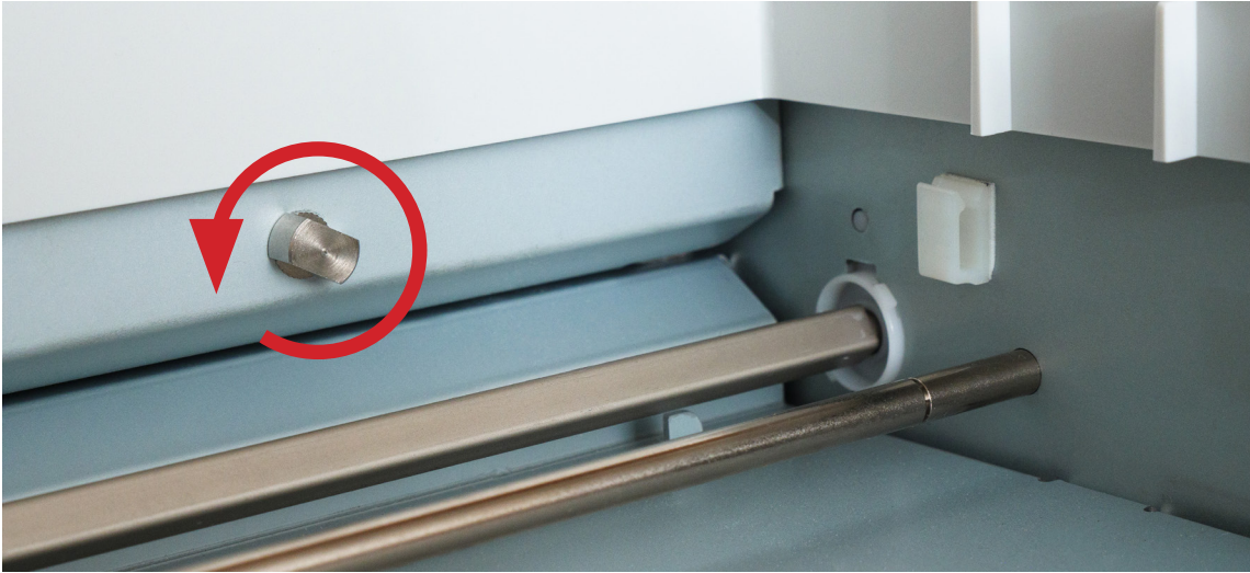
Image 1: Shows the shipping bolt and location
