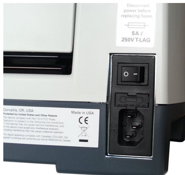
Image 3: Shows the power module in the back of the embosser
