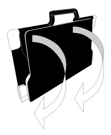
**2.** Unfold the top panel until it is roughly parallel with the lower panel.
