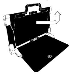
3. Hold your tablet with the screen side facing you, making sure the HumanWare logo is at the top. Carefully insert the top of your tablet into the slot and slide it forward until you reach the back end of the slot. Push the bottom part of the
